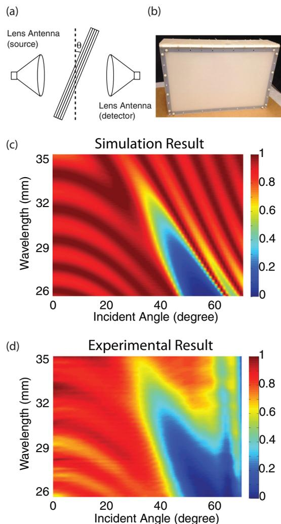
FIG. 5. (Color online) Experimental verification. (a) A schematic illustration of the experimental setup. (b) Photo of the fabricated sample. (c), (d) Comparison between  $p$ -polarized transmission spectrum of transfer matrix method and the experimental measurements.
