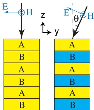
FIG. 1. (Color online) Effective index for  $p$ -polarized light in an isotropic (A)-anisotropic (B) multilayer system. Left panel: all the layers have the same index. Right panel: the change in incident angle leads to a change in the index of the anisotropic (B) material layers.
