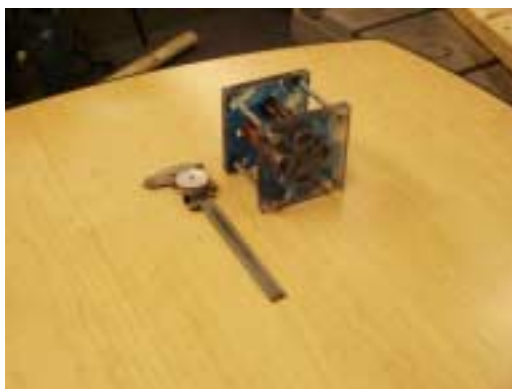
Figure 6: A Nearly Complete Cold Flow MCRI Engine
