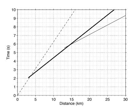
Figure 1: Travel times of direct and head waves obtained from the two-layer model.
