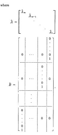
Each  $\hat{A}_k(k = 1, 2, \dots, m)$  is a companion matrix corresponding to the eigenvalues influenced by  $b_k$ . This class of systems has a unique representation except for the orde ing of the  $A_k$ . A typical submatrix  $A_k$  of A is given by
