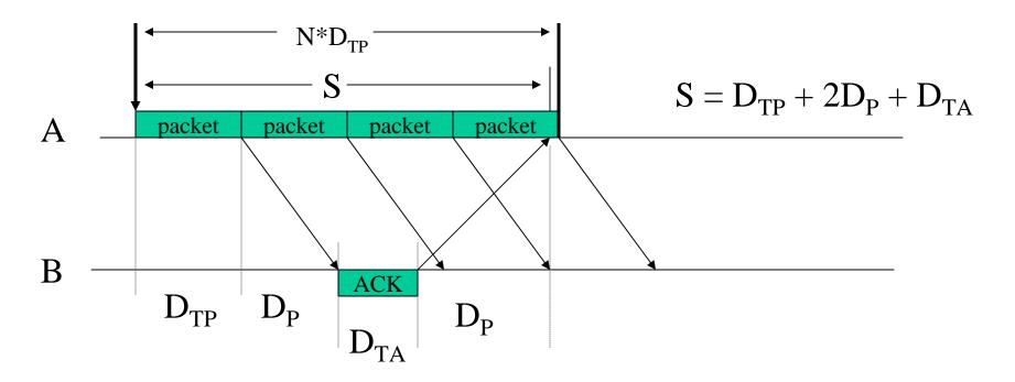
We want to choose N large enough to allow continuous transmission while waiting for an ACK for the first packet of the window,
