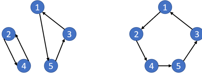
Figure 1: Two cycle covers for a graph with 5 vertices, corresponding to permutation (1, 5, 3), (2, 4) and permutation (1, 2, 4, 5, 3) .
