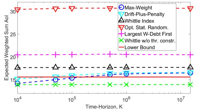
Fig. 2. Performance of a network with size  $M = 15$  over time. Notice that the abscissa is scaled logarithmically.
