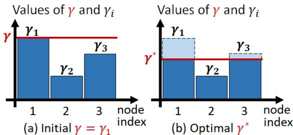
Fig. 1. Illustration of Algorithm 1 in a network with 3 nodes. On the left, the initial configuration with  $\gamma = \max\{\gamma_i\}$ . On the right, the outcome  $\gamma^*$  implies that under policy  $R^*$  node 2 will operate with minimum required scheduling probability  $\mu_2 = q_2/p_2$ , while the other two nodes will operate with a scheduling probability that is larger than the minimum.
