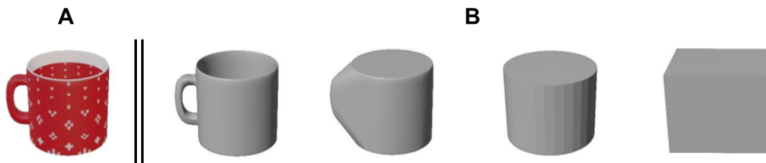
Figure 1: Different representations for rendering and physical interactions. (A) “Shape” is used for rendering an object onto the screen. (B) “Body” is an approximation used to determine collisions, apply forces, and track objects. Example approximations are shown in increasing coarseness from left to right: mesh collider, convex hull, cylinder collider, bounding box.
