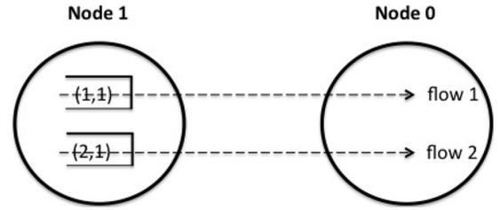
Fig. 1. Single-server system with two parallel queues, cast as a multihop network. Traffic flow 1 is heavy-tailed, and traffic flow 2 is light-tailed. Since the network has single-hop traffic, the Back-Pressure policy reduces to Max-Weight scheduling. The findings of [15] imply that the light-tailed flow is delay unstable.
