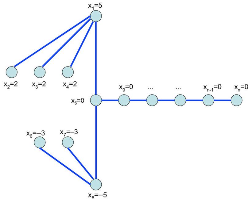
Fig. 1. A connected graph on  $n$  nodes showing that  $V(x)$  is not a Lyapunov function when  $n \geq 8$ . All arcs of the form  $(i, i)$  are also assumed to be present, but are not shown. The nodes perform an iteration of the symmetric, equal-neighbor model according to this graph.
