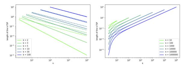
Figure 3 Convergence rate of the length of the *k*-TSP  $\Theta\left((k-1)/n^{\frac{1}{2}\left(1+\frac{1}{k-1}\right)}\right)$  (in solid lines) compared to the rate of convergence of the simple heuristic  $\Theta((k-1)/\sqrt{n})$  (in dashed lines), as a function of *n* and *k*.
