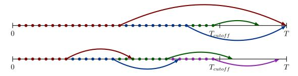
Figure 1 Consolidation-driven dispatch based on order deadlines from the TSP approximation (top), versus dispersion-driven dispatch based on customer wait times from the TRP approximation (bottom) for m = 4 vehicles.
