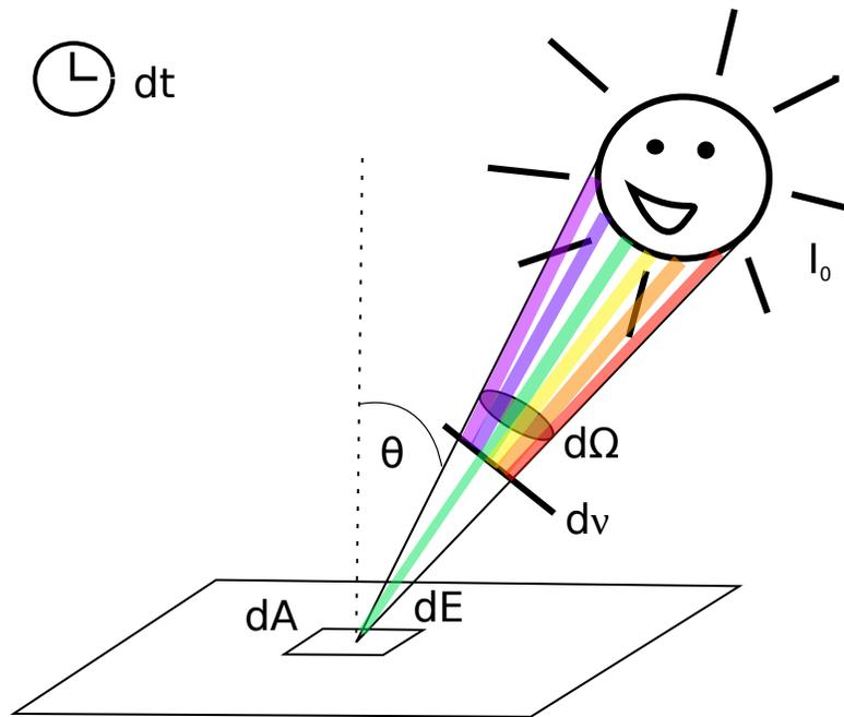
Figure 5: Description of the energy detected at a location in space for a period of time  $dt$  over an area  $dA$  arriving at an angle  $\theta$  from an object with intensity  $I_0$ , an angular size  $d\Omega$ , through a frequency range  $d\nu$  (in this case, only the green light).
