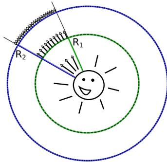
Figure 6: A depiction of the flux detected from our sun as a function of distance from the sun. Imagining shells that fully enclose the sun, we know that the energy passing through each shell per unit time must be the same (equal to the total luminosity of the sun). As a result, the flux must be less in the larger outer shell: reduced proportional to  $1/d^2$
