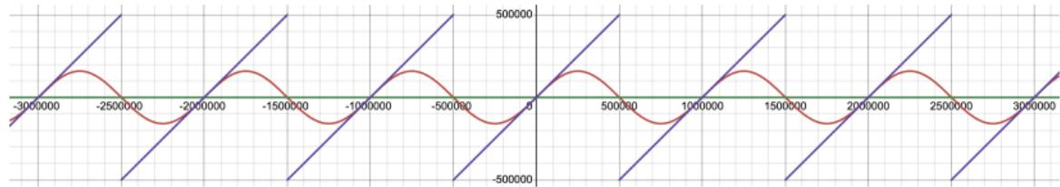
Fix: approximate the scaled sine function with period  $10^{12}$  using its Taylor series. Then evaluate the Taylor series on the ciphertext.
