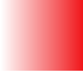
Figure 13: A varying temperature field. Here the gradient points in the \hat{x} direction; derivatives of T in other directions will be smaller in magnitude.
