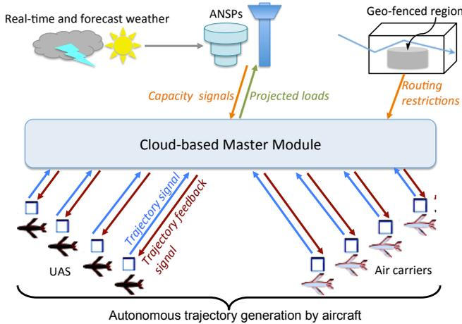
Figure 5: High-level depiction of the DRIFT architecture.
