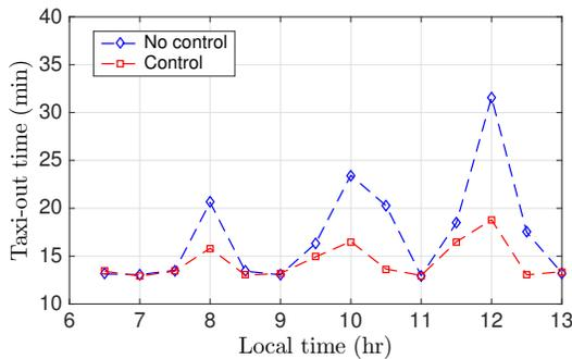
Fig. 14. Comparison of the averaged taxi-out time obtained using the receding horizon control policy
