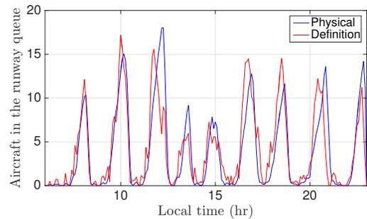
Fig. 4. Comparison of the total queue length obtained from the definition of the runway queue, and the physical queue observed at the airport for a typical day.
