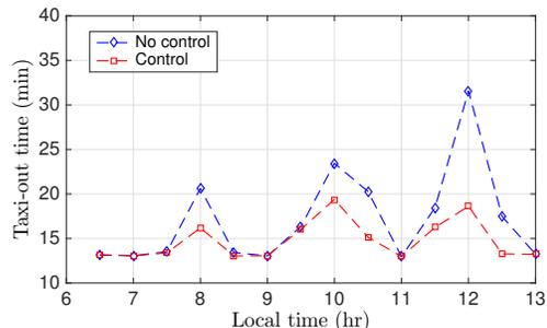
Fig. 12. A comparison between the mean taxi-out time (30-min average) obtained using the pushback control policy, and when aircraft pushback without any gate-holds.
