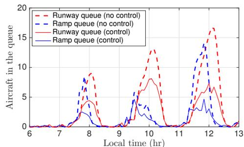
Fig. 11. Comparison of the number of flights in the ramp and runway queues with, and without, the optimal pushback policy.
