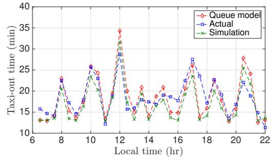
Fig. 8. Comparison of the taxi-out times (averaged over a 30-min window) obtained from the tandem queue model, actual data and simulations for a typical day.
