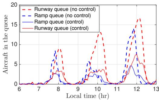
Fig. 13. Comparison of the number of flights in the queue obtained using the receding horizon control policy.
