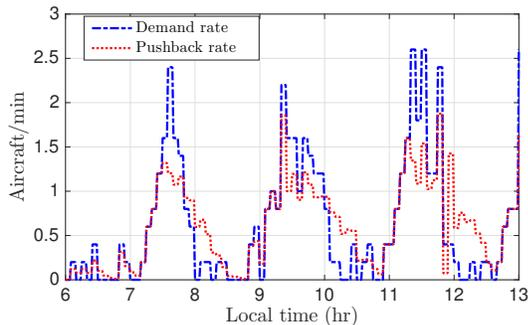
Fig. 9. Variation of the optimal pushback rate (aircraft/min) for a given demand profile on a typical day.
