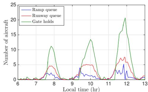
Fig. 10. The number of aircraft in the ramp queue ( $x_1$ ), runway queue ( $x_2$ ), and gate holds ( $h$ ) with the optimal push back policy.
