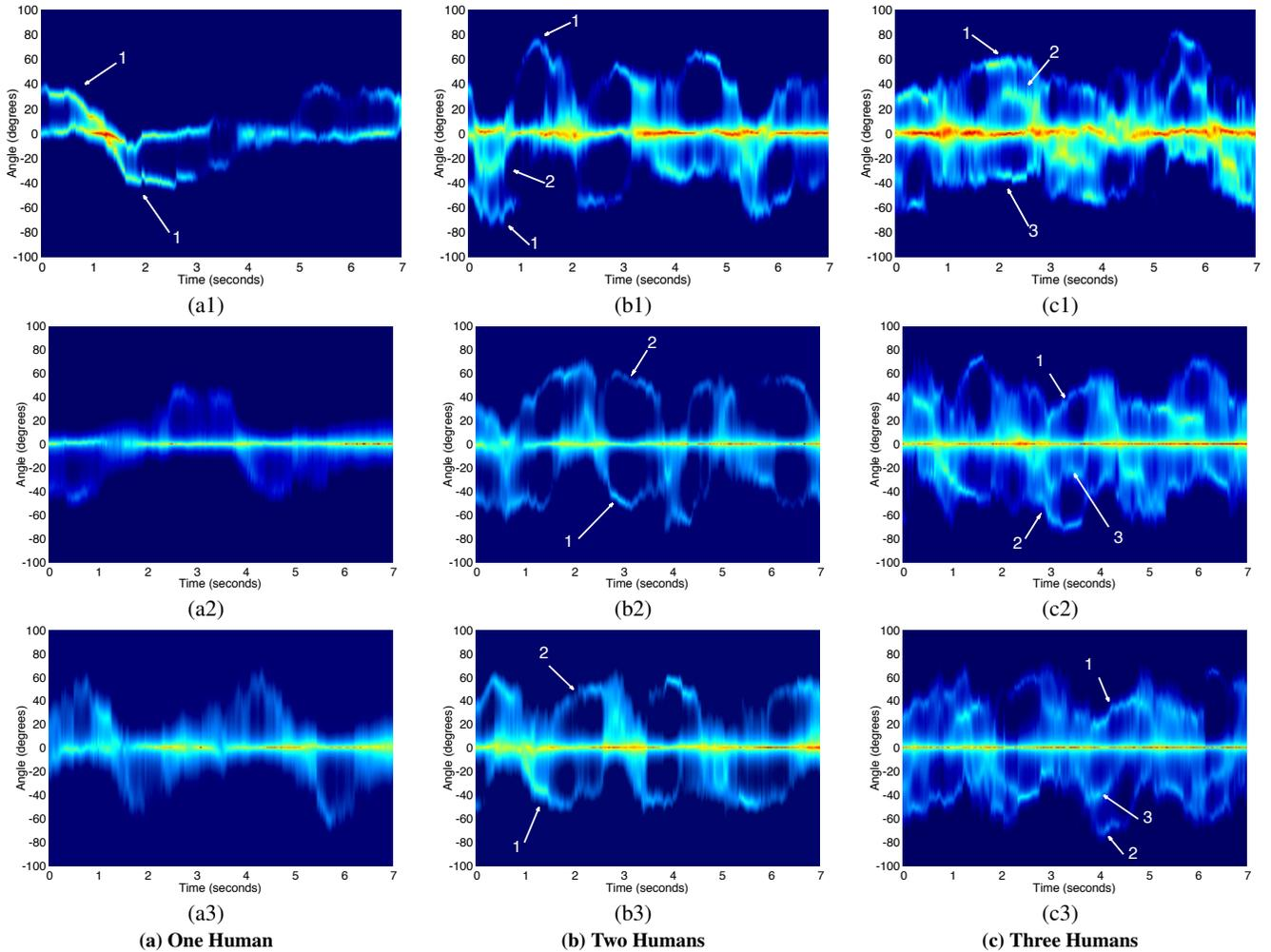
**Figure 8—Tracking human motion with Wi-Vi.** The figures show output traces with a different number of humans after processing with the smoothed MUSIC algorithm. They plot  $A'[\theta, n]$  where  $\theta$  is the angle in  $[-90, 90]$  is plotted on the y-axis and time is on the x-axis. (a) shows traces for one human; (b) for two humans; and (c) for three humans moving behind the wall of a closed room.
