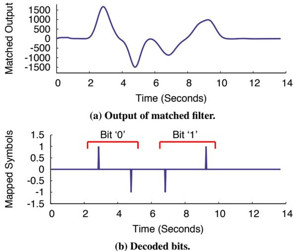
**Figure 7—Gesture Decoding in Wi-Vi.** The figure shows how Wi-Vi decodes the gestures of Fig. 5. (a) shows the output of the matched filter step. (b) shows the output of the peak detector. The sequence  $(1, -1)$  represents bit ‘0’, whereas the sequence  $(-1, 1)$  represents bit ‘1’.
