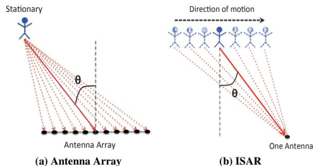
**Figure 1—A Moving Object as an Antenna Array.** In (a), an antenna array is able to locate an object by steering its beam spatially. In (b), the moving object itself emulates an antenna array; hence, it acts as an inverse synthetic aperture. Wi-Vi leverages this principle in order to beamform the received signal in time (rather than in space) and locate the moving object.
