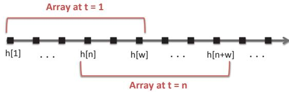
**Figure 2—Time samples as Antenna Arrays.** Wi-Vi groups consecutive time samples into overlapping windows of size  $w$ , then treats each window  $h[n] \dots h[n+w]$  as an antenna array. This allows it to track the direction of a moving object with respect to the receiver.
