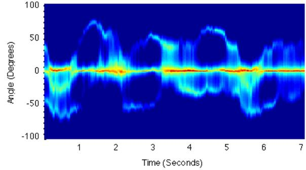
**Figure 4—Wi-Vi tracks the motion of two humans.** The figure shows how the presence of two humans translates into two curved lines whose angles vary in time, and one straight line which corresponds to the DC.
