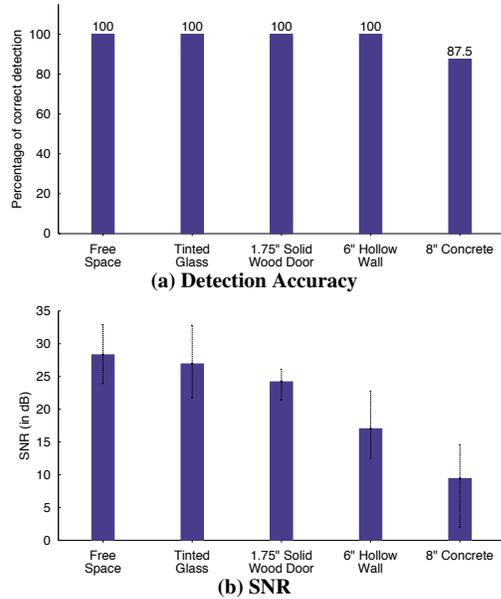
**Figure 12—Gesture detection in different building structures.** (a) plots the detection accuracy of Wi-Vi for different types of obstructions. (b) shows the average SNR of the experiments done through these different materials, with the error bars showing the minimum and maximum achieved SNRs across the trials.
