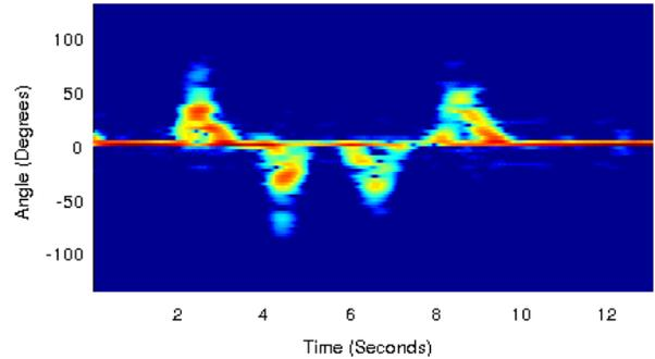
**Figure 5—Gestures as detected by Wi-Vi.** The figure shows a sequence of four steps: step forward, step backward, step backward, step forward. Forward steps appear as triangles above the zero line; backward steps appear as inverted triangles below the zero line. Each pair of steps represents a gesture/bit: the first two represent bit ‘0’, the second two represent bit ‘1’.
