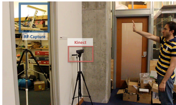
Figure 6-12: Tracking the Human Hand Through Walls. RF-Capture tracks the subject's palm through a wall while the Kinect tracks it in line-of-sight.
