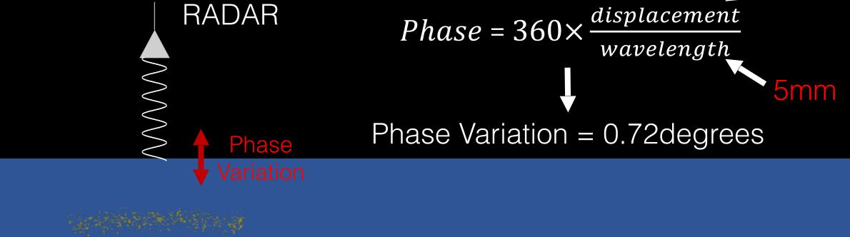
The phase of the milimeter-wave RADAR encodes transmitted information from underwater
