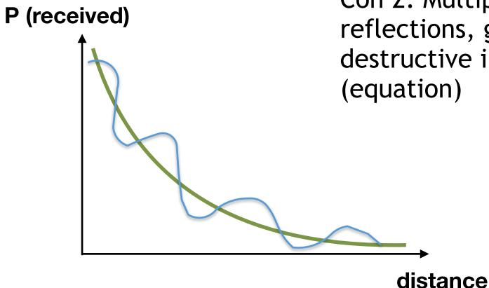
Con 2: Multipath: Due to reflections, get constructive and destructive interference (equation)
