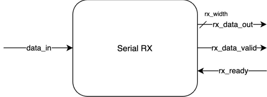
Figure 6: Serial RX module inputs and outputs
