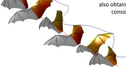
In order to understand the advantages and disadvantages of flapping flight we are developing the computational capabilities to analyze and design flapping-wing flight vehicles. The procedure incorporates a multi-fidelity toolset, starting with a simple wake-only analysis and ending with validation and refinement using full-blown Computational Fluid Dynamics (CFD).
