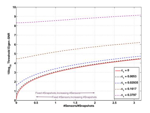
Figure 1: Plot of the minimum (generalized) Eigen-SNR required (given by (12)) to be able to asymptotically discriminate between the "signal" and "noise" eigenvalue of the matrix  $\widehat{\mathbf{R}}_{\widehat{\Sigma}}$  constructed as in (8) as a function of the ratio of the number of sensors to snapshots for different values of  $c_1 \approx$ Number of sensors/Number of noise-only snapshots.
