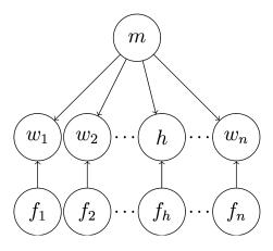
Fig. 1. Graphical representation of a generative model of a sentence. If the indicator variable  $f_i$  has value 1,  $w_t$  is generated based on semantic relatedness to the sentence meaning m; otherwise,  $w_t$  is sampled from a trigram language model based on the immediately preceding two words.
