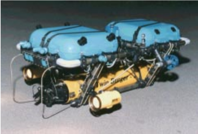
Fig. 9 Twin-Burger 1: the versatile underwater robot testbed
