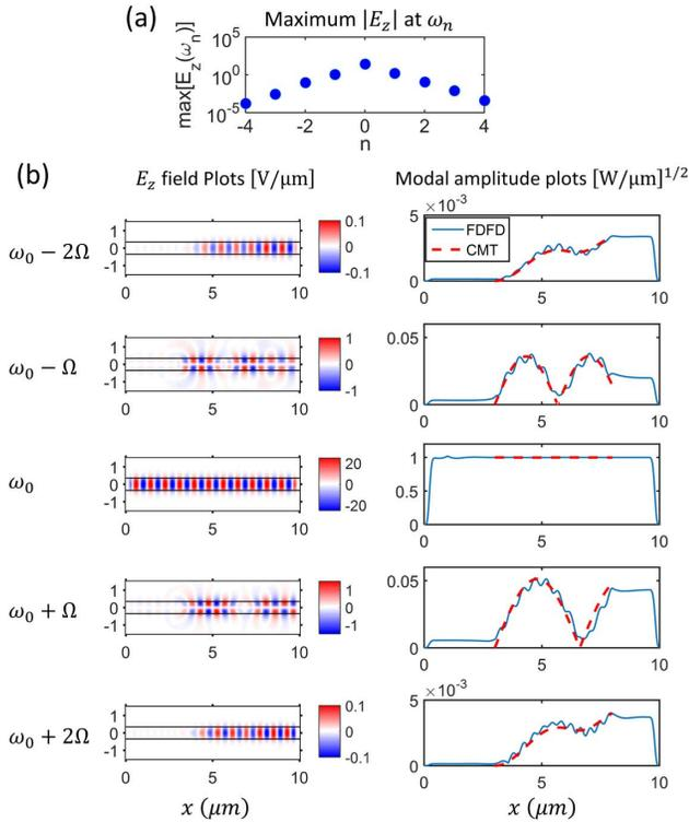
**Fig. 2.** (a) Plot of maximum field amplitude that exists in each frequency sideband as indexed with  $n$ . The field amplitude decreases exponentially with  $n$ . (b) (left) Field profiles of frequency components with  $n \in [-2, 2]$  and (right) comparison of the MF-FDFD results with coupled mode theory (CMT).
