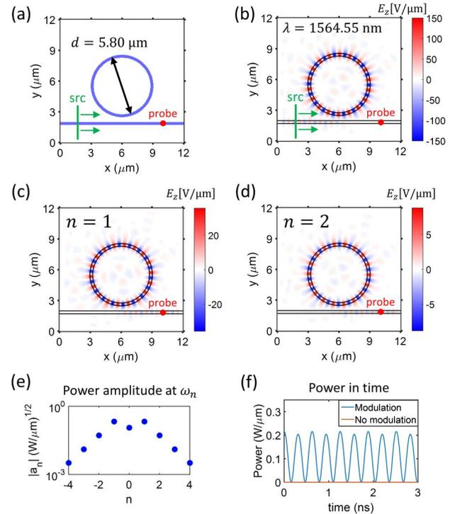
**Fig. 3.** (a) Schematic of the ring resonator geometry. (b) At  $\lambda = 1564.55 \text{ nm}$ , the  $\text{TE}_0$  mode from the waveguide is critically coupled to the ring resonator. (c), (d) Field profiles for waves at the  $n = 1, 2$  sidebands, respectively. The power inside the ring at these sidebands is coupled to the waveguide and can be detected at the probe. (e) Power amplitude at the probe at each frequency. (f) Plot of power at the probe as a function of time.
