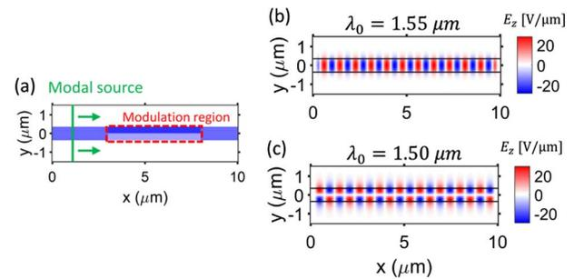
**Fig. 1.** (a) Schematic of the waveguide structure with the source location and modulation region indicated. In the modulation region, the top and bottom halves of the waveguide are modulated with a relative phase difference of  $\pi$ . (b), (c) Modal profiles of the  $\text{TE}_0$  and  $\text{TE}_1$  modes of the waveguide at  $\lambda_0 = 1.55 \mu\text{m}$  and  $\lambda_1 = 1.50 \mu\text{m}$ , respectively. Both modes carry a guided power normalized to 1 W/ $\mu\text{m}$ .
