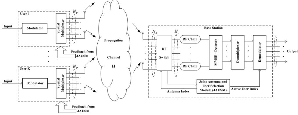
Fig. 1. Block diagram of the uplink multiuser MIMO system.
