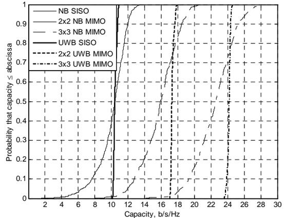
Fig. 7 Capacity of narrowband and UWB SISO and MIMO for LOS
