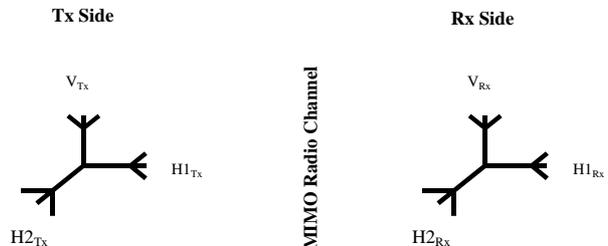
Fig. 1. Tri-polarized MIMO antenna configuration
