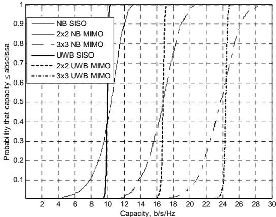
Fig. 6 Capacity of narrowband and UWB SISO and MIMO for NLOS
