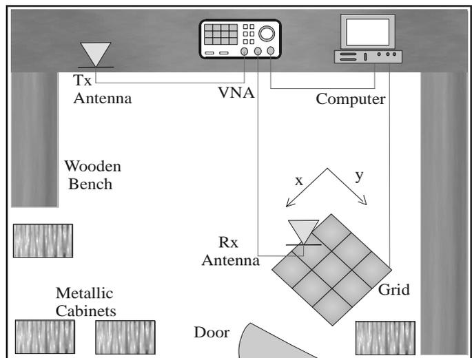
Fig. 2 Schematic of VNA measurement system
