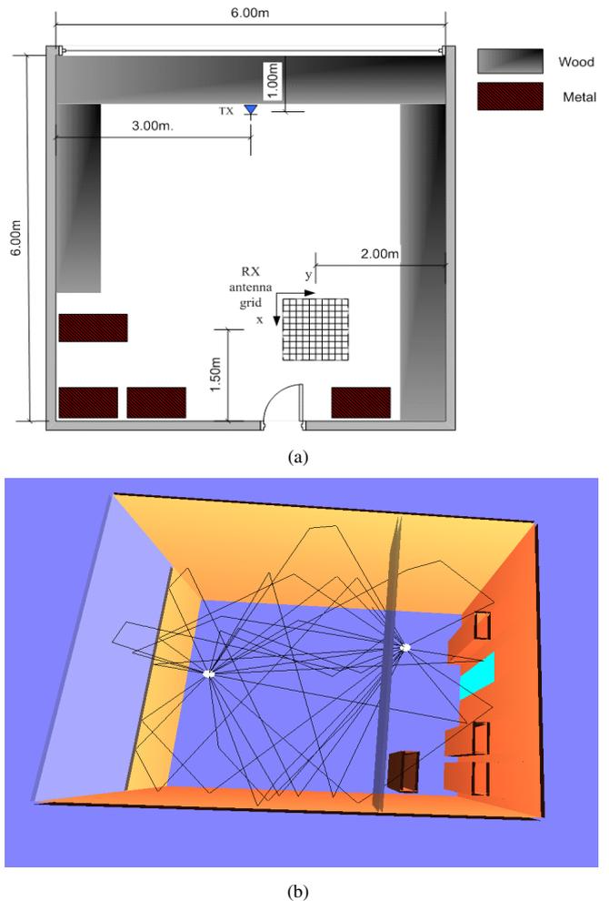
Fig. 2. The ray-tracing simulation: (a) a plan view of the simulated indoor propagation environment, and (b) three-dimensional visualization of the ray paths at the center of the receiving grid.
