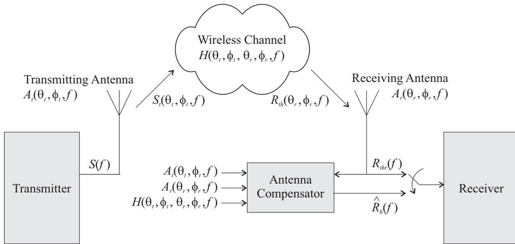
Fig. 1. Angularly asymmetric signal distortion is caused to the UWB signal,  $S(f)$ , due to the antennas in a multipath environment. The antenna compensator equalizes the antenna distortion – only at the receiver in the case illustrated here.
