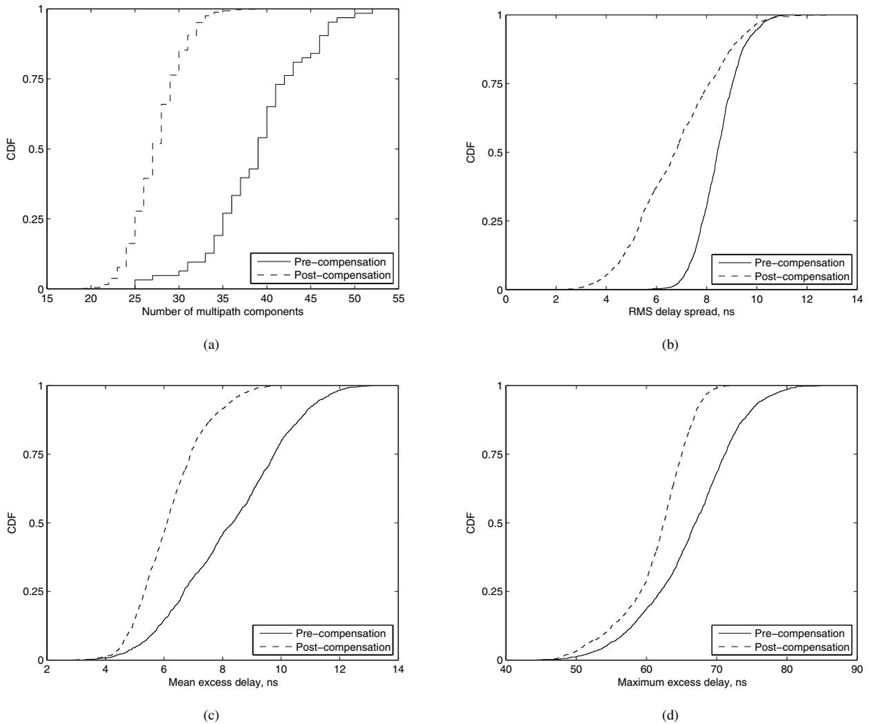
Fig. 3. The pre- and post-compensation cumulative distribution functions (CDFs) of the (a) number of multipath components, (b) rms delay spread, (c) mean excess delay, and (d) maximum excess delay.
