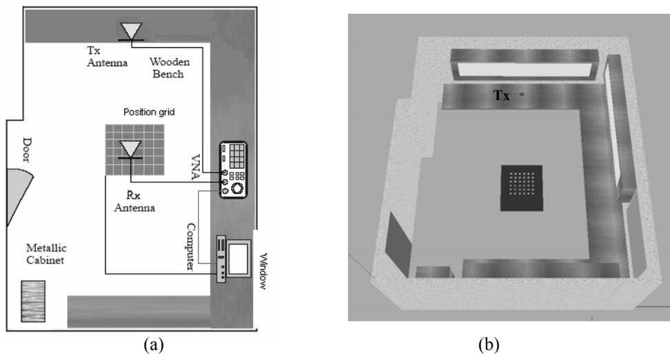
**Fig. 1** a)- A plan view of the measurement environment: the room is 5m×4.7m×2.6m, the transmitter (Tx) and the receivers are located at the same height of 1.35 m. b)- Pictorial view of the RT reconstructed scenario (ceiling not shown); the transmitter and the receivers (white dots grid) are also shown.
