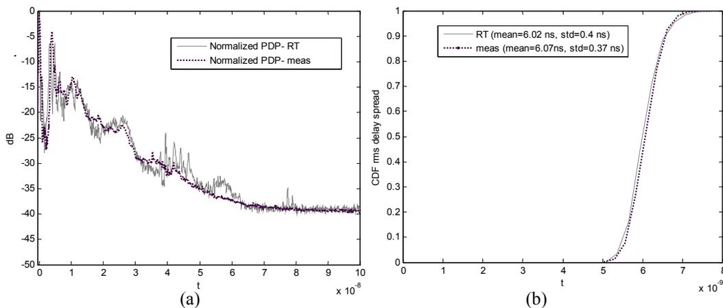
**Figs. 2** a)- Comparison of the PDPs (measured and simulated). The abscissa indicates the time exceeding that of the first arrived ray. b)- Cumulative Distribution Function (CDF) of the *rms* delay spread (measured and simulated).
