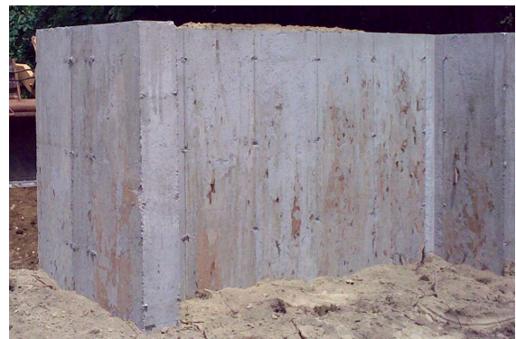
Fig. 12. The 10 cm thick solid concrete test wall.
