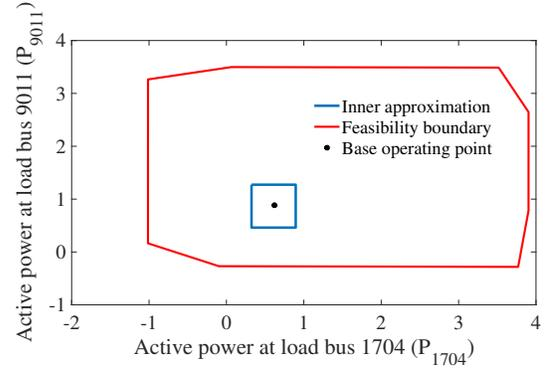
Fig. 5. Feasibility set of an OPF for 1354-bus medium part of European system
