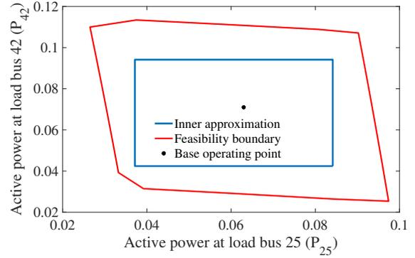
Fig. 3. Feasibility set of an OPF for IEEE 57-bus system
