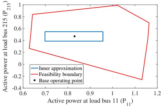
Fig. 4. Feasibility set of an OPF for IEEE 300-bus system
