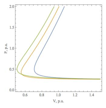
Fig. 1. Dependence of the total power consumption P on voltage at bus 1 for  $P_L = 0.25 \, p.u., Q_L = 0.25 \, p.u.$  (blue),  $P_L = 0.25 \, p.u., Q_L = 0.25 \, p.u.$  $0.0 \, p.u.$  (orange),  $P_L = 0.25 \, p.u.$ ,  $Q_L = -0.25 \, p.u.$  (green).
