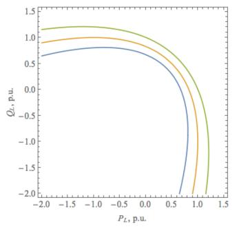
Fig. 2. Lodability limit boundaries defined by equation (19) with V = $0.9 \, p.u.$  (blue),  $V = 1.0 \, p.u.$  (orange),  $V = 1.1 \, p.u.$  (green).
