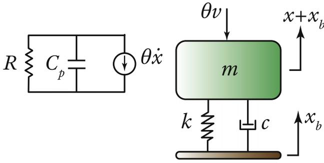
**Figure 1.** A base-excited PEH modeled as an SDOF oscillator coupled with an electric circuit modeling a load resistance and the inherent capacitance of the piezoelectric layer.
