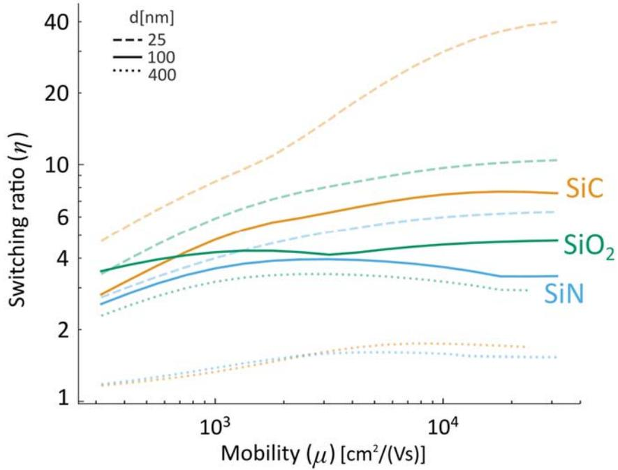
**Fig 6.** Thermal switching between parallel graphene sheets (Fig. 1a), now on identical substrates that support surface phonon-polaritons (SiC, SiN, or SiO<sub>2</sub>). Different line styles indicate the switching ratio  $\eta$  for separation distance  $d$  of 25 nm (dashed), 100 nm (solid), and 400 nm (dotted) ( $T=300$  K). As before, for each value of mobility, the respective Fermi levels for the ON ( $E_{1,2}^{\text{on}}$ ) and the OFF ( $E_{1,2}^{\text{off}}$ ) state are determined.
