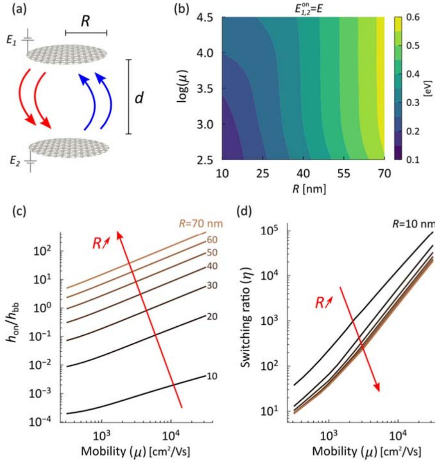
**Fig 4.** Radiative thermal switching between parallel graphene disks (a). Optimal carrier concentration levels  $E_{1,2}^{\text{on}} = E$  for the “ON” state (b), RHT enhancement (c), and the switching ratio (d), as a function of mobility ( $\mu$ ) and disk radius ( $R$ ). Here,  $T = 300$  K,  $d = 200$  nm.
