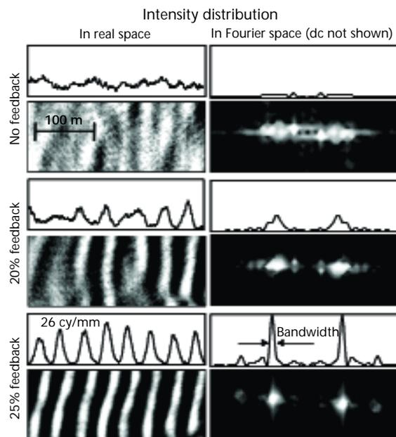
**Figure 1.** Experimental results, showing pattern formation in a temporally incoherent nonlinear optical cavity, displaying the narrowing of the spatial spectrum of the pattern with increasing feedback intensity. Shown are photographs of the intensity distribution along with their calculated spatial (Fourier) power spectrum (*right*), at various feedback values. The bandwidth narrowing is obvious in these pictures as the stripes become sharper and more regular with increasing feedback.
