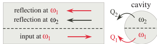
Fig. 4. Schematic diagram of waveguide-cavity system. Input light from a waveguide (left) at one frequency \omega_1 is coupled to a doubly-resonant cavity (with resonances at \omega_1 and \omega_2 , with respective lifetimes Q_1 and Q_2 ) and converted to a cavity mode at another frequency \omega_2 by a \chi^{(2)} process. The converted light is radiated back into the waveguide at both frequencies.
