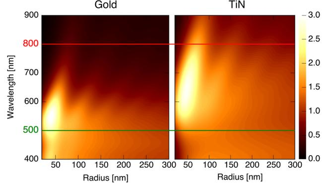
**Figure 2.** Absorption efficiency as a function of wavelength and radius for a homogeneous gold (left) and titanium-nitride (right) spherical particle, in water. Values obtained from Mie scattering equations. Highlighted green (500 nm) and red (800 nm) lines correspond to the two wavelengths used for selective heating of the two hemispheres of the composite asymmetric particle (Figure 1a).
