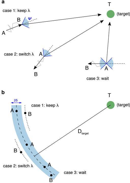
**Figure 4.** Scheme for guiding the composite asymmetric particle: the particle, that in the short time interval  $\tau_1$  moves from A to B, can be guided to the target location (T) either when its location is known (a) or when only the distance to the target is known (b).
