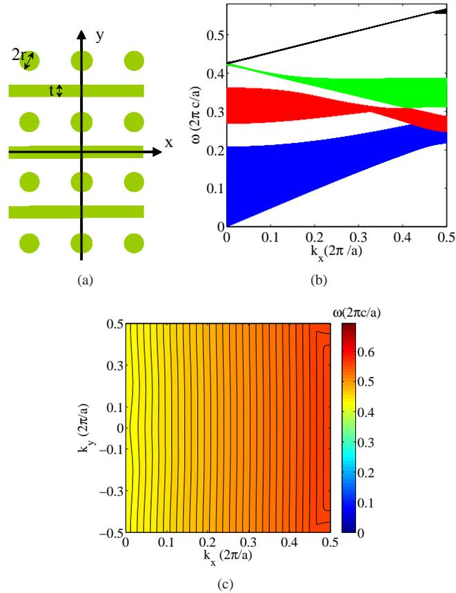
Fig. 2. Proposed 2D PhC structure (a) Schematic of the refractive index: the rods, of radius  $r$ , and waveguides, of thickness  $t$ , (shown in green) both have  $n = 3.5$ , and are surrounded by air ( $n = 1$ ). The rods form a square lattice, with lattice constant  $a$ , and the waveguides are halfway (on the  $y$ -axis) between the rods. (b) Projected band diagram of lowest four TM bands for  $r = 0.16a$  and  $t = 0.2a$ . (c) Color contour plot of the frequency of the fourth TM band.
