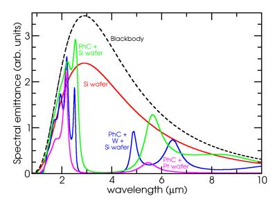
Fig. 4. Spectral emittance of four structures at 1000 K: a polished Si wafer (Fig. 3(a)), a polished Si wafer with a 4-bilayer 1D PhC (Fig. 3(b)), a polished Si wafer with tungsten and a 4-bilayer 1D PhC (Fig. 3(c)), and a platinum wafer with a 3-bilayer 1D PhC (similar to Fig. 3(c)). The efficiency, power, and overall figure of merit for each structure is listed in Table 2.
