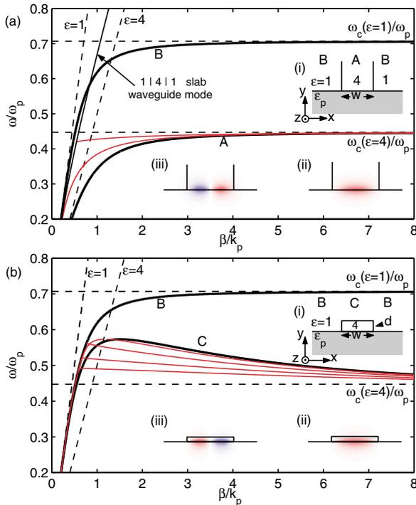
FIG. 3 (color).  $\omega$ - $\beta$  diagrams (red curves) for SP-based waveguide structures [insets (i)] with  $w/\lambda_p = 0.25$  and  $d/\lambda_p = 0.02$  and the  $H_x$  component of their first two modes at (a)  $\omega/\omega_p = 0.444$  and (b)  $\omega/\omega_p = 0.47$  [insets (ii) and (iii)].
