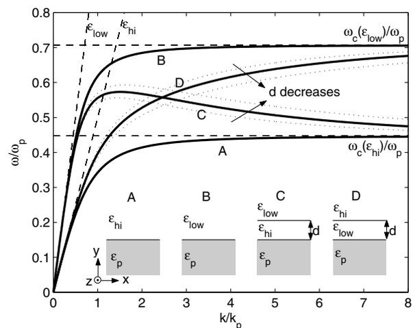
FIG. 1.  $\omega$ - $k$  diagrams (solid curves) for conventional layered surface-plasmon structures (insets A–D) with  $\epsilon_{hi} = 4$  and  $\epsilon_{low} = 1$  (air). Layer thicknesses  $d/\lambda_p = 0.015, 0.02,$  and  $0.025$  are used for C and D (solid + dotted curves). The light lines  $\omega/\omega_p = \sqrt{\epsilon}k/k_p$  (“vertical” dashed lines) and the cutoff frequencies  $\omega_c(\epsilon)/\omega_p = 1/\sqrt{1 + \epsilon}$  (horizontal dashed lines) are shown.
