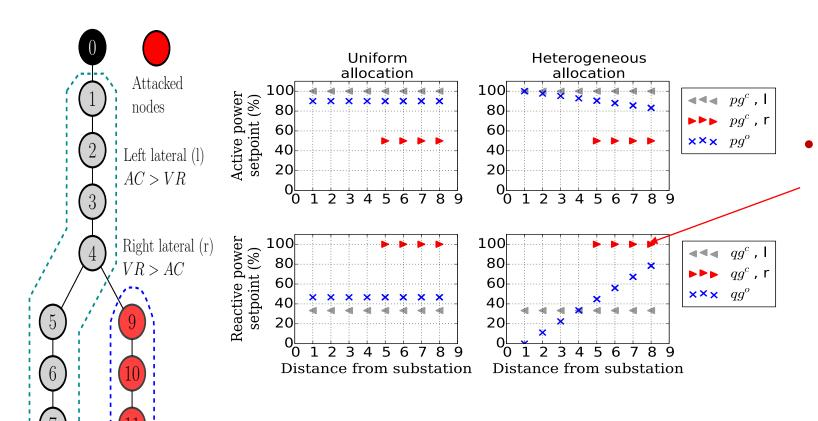
Diversification holds for "heterogeneous allocation" with downstream DERs with more reactive power
