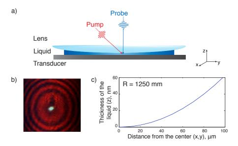
Figure 3.7. (a) Sketch of the flat-curved sample cell configuration. (b) Recorded image showing the Newton's interference rings. (c) Variation of the liquid film thickness at different lateral positions. The thickness variation is very small close to the center and rapidly increases away from the contact zone.
