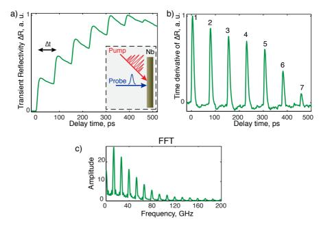
Figure 2.10. (a)Example of a normalized time domain reflectivity signal obtained with the pulse shaper. The optical pulse sequence was focused on Niobium thin film. The time difference between the individual pulses was arbitrarily adjusted to  $\Delta t \sim 75$  ps. (b) Time derivative of the measured signal. (c) Frequency spectrum of the reflectivity signal.
