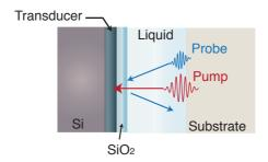
Figure 4.11. Schematic of the multilayer sample. A thin  $SiO_2$  capping layer is introduced in order to thermally insulate the liquid from the laser heated Cr metallic transducer film. As before, a transparent glass cover substrate and glycerol was used in this specific sample configuration.
