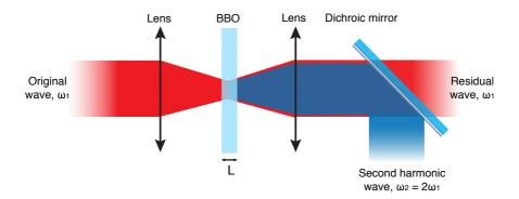
Figure 2.11. Illustration of the optical second harmonic generation process. An incident beam at a wavelength of 790 nm is focused into a BBO crystal. A fraction of the incident light is converted into light at the double frequency, leading to a blue beam at a wavelength of 395 nm. The 395 nm light is then filtered out.
