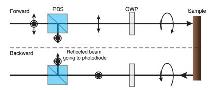
Figure 2.12. Brief illustration of the polarisation change occurring with the combination of a PBS and a quarter waveplate. The transmitted light from the PBS passes through the quarter waveplate, changing its polarization from linear to circular and reflects from the sample. After passing twice through the quarter waveplate, the probe polarization direction becomes vertical and the probe is reflected by the PBS.
