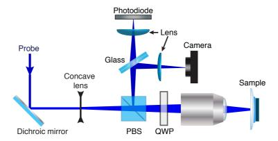
Figure 2.14. Scheme of the 2D imaging setup that use the femtosecond probe beam for illumination.
