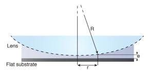
Figure 3.5. The curved-flat experimental setup of the Newton's rings. The liquid is squeezed in between the curved surface and the flat surface.
