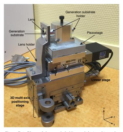
Figure B.1. Photo of the sample holder used during this work.
