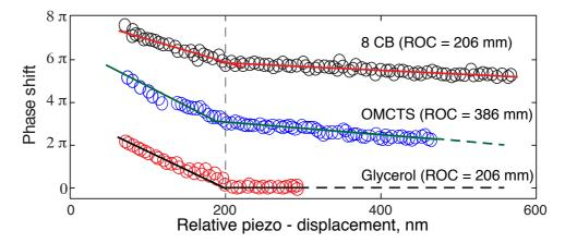
Figure 5.16. Phase shifts of the 46 GHz Brillouin oscillations in the glass lens at different piezostage displacements, extracted from Brillouin scattering data for three investigated liquids, glycerol, OMCTS and 8 CB.
