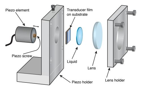
Figure B.2. Schematic representation of the first version of the sample configuration tested during this work. The Piezo actuator is a cylinder on which a screw glued with the generation substrate is attached. The liquid drop is squeezed in between the transducer film substrate and the lens.
