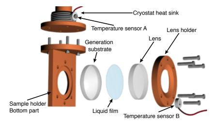
Figure 4.4. Sketch of the sample holder designed for use in a cryostat chamber. The liquid is squeezed between two substrates - flat generation substrate and the lens which are placed in a copper holder. The whole construction is attached to a heat sink of a cryostat. Two temperature sensors are placed to control the temperature of the cryostat chamber (sensor A) and of the sample (sensor B). Reprint from [86].
