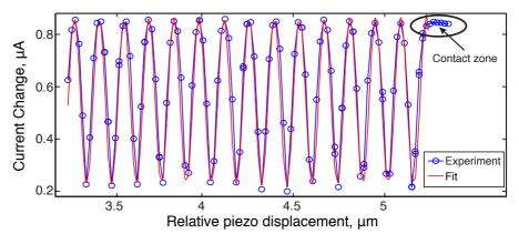
Figure B.5. Change of the reflected probe intensity from different thicknesses of glycerol. The sample configuration consists of a silicon substrate holding a 50 nm thick Chromium film, glycerol, and an AR plano - convex lens. This sort of measurement allows to optically determine the zone where lens is in direct contact with the flat generation substrate (black ellipse). From the spatial period of the oscillations, the refractive index of the liquid may be calculated.
