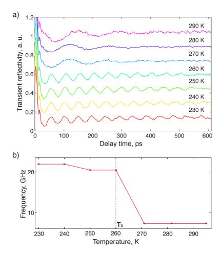
Figure 4.5. (a) Time derivative of recorded transient reflectivity signals obtained with OMCTS at different temperatures and at a given pump fluence  $0.75~\mathrm{mJ.cm^{-2}}$ . The time derivative was taken for better display. (b) Temperature dependent Brillouin frequency. T  $_x$  indicates the liquid to crystalline phase transition temperature.
