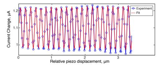
Figure B.6. Change of the reflected probe intensity from different thicknesses of OM-CTS. The sample configuration consists of a silicon substrate holding a 50 nm thick Chromium film, OMCTS, and an uncoated plano-convex lens. From the spatial period of the oscillations, the refractive index n of OMCTS at the probe wave length is extracted.
