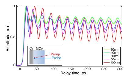
Figure 2.4. Transient reflectivity change of several  $Cr/SiO_2$  samples of different Cr thicknesses. The inset shows the experimental single layer system. Upon laser generation in the Cr film, the acoustic strain is transmitted into the adjacent  $SiO_2$  substrate where it is detected by delayed light probe pulses through Brillouin light scattering. The time oscillations at the frequency f=41 GHz correspond to the Brillouin frequency in  $SiO_2$ .
