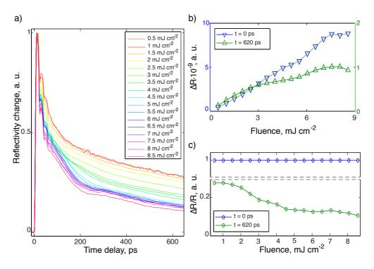
Figure 4.3. (a) Normalized transient reflectivity signals obtained in the configuration depicted in Fig. 4.2 at different pump fluences. The shape of the signals varies depending on the pump fluence due to the nonlinear laser excitation and thermalization process. Fluence dependence of the raw (a) or normalized (b) transient reflectivity signals at 0 ps and 620 ps.
