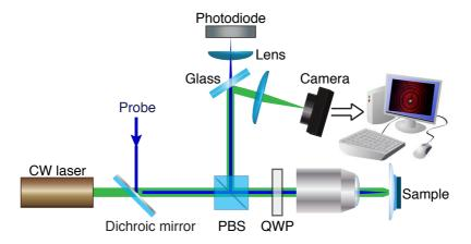
Figure 2.13. Simplified scheme of the simple 2D imaging setup. The collimated laser module illuminates the sample surface which is imaged in the CMOS camera.
