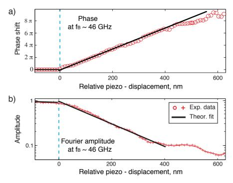
Figure 5.5. Fourier phase shift (a) and amplitude (b) of the 46 GHz Brillouin oscillations in glass, extracted from TDBS piezo measurements with Glycerol. The raw data are presented in Fig. 5.4.
