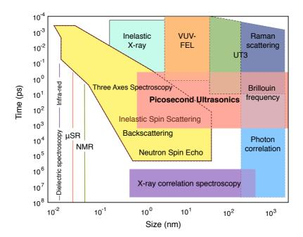
Figure 1.3. Graphical representation of the experimental techniques used for investigation of atomic, molecular, crystalline structure of materials. (VUV-FEL - Vacuum UltraViolet Free Electron Laser; UT3 - Ultrasonic Testing Tandem Technique; NMR - Nuclear Magnetic Resonance;  $\mu$ SR - Muon Spin Rotation).
