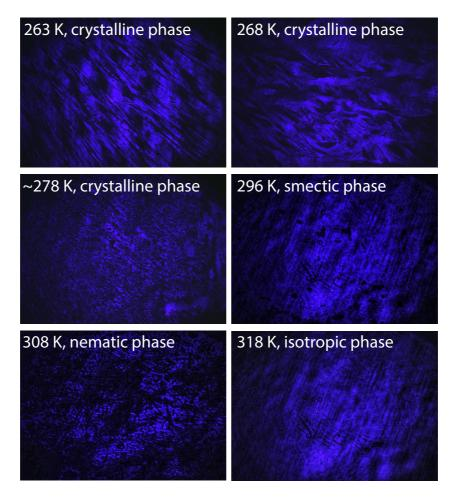
Figure 5.13. Example of images showing the 8 CB texture at various temperatures. The images were obtained using the 2D imaging technique.
