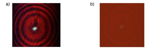
Figure B.3. Images of the sample surfaces obtained from a sample configuration with a Chromium transducer film on a flat silicon substrate, glycerol, and either a lens with antireflection coating (a) or a lens without antireflection coating (b). The Newton's rings are well contrasted in (a) and undetectable in (b).
