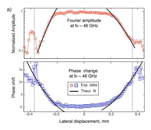
Figure 5.7. (a) Normalized acoustic amplitude and (b) phase shifts of the 46 GHz signal oscillations extracted from Brillouin scattering in the lens (see raw data in Fig. 5.6 (a)). The extracted amplitude and phase shift provide information on the acoustic attenuation coefficient  $\alpha$  and the sound velocity  $c_l$  in OMCTS.
