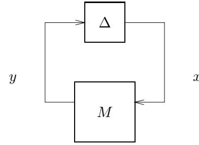
Figure 6.1: Plant  $M$  and uncertainty diagonal structure  $\Delta$ .
