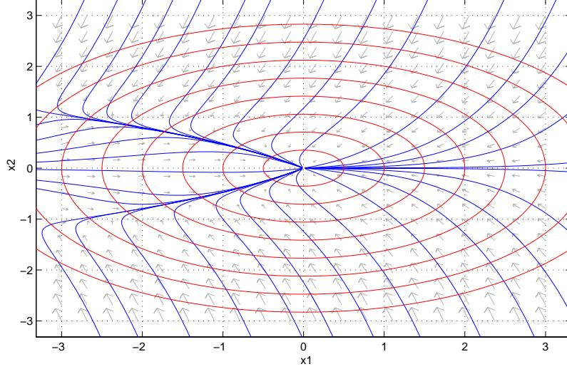
Figure 7.1: Phase plot and Lyapunov function level sets.
