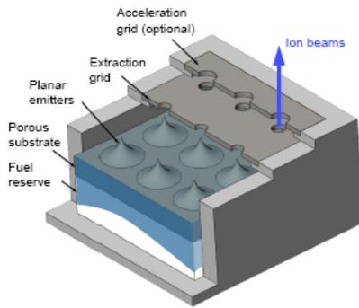
Figure 1: Schematic of the electro spray thruster.
