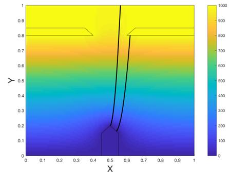
Figure 2: Ion trajectory for ideal release point.
