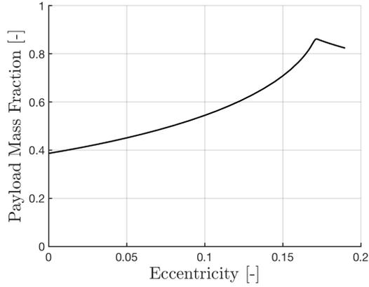
Figure 6: Payload mass fraction versus eccentricity for a semi-major axis of 1.21au.
