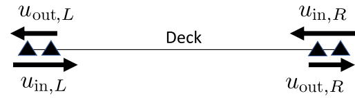
Figure 8. Decomposition of the wavefield propagating through a deck into incoming and outgoing waves at two locations of the deck. Triangles indicate the location of accelerometers. The color version of this figure is available only in the electronic edition.
