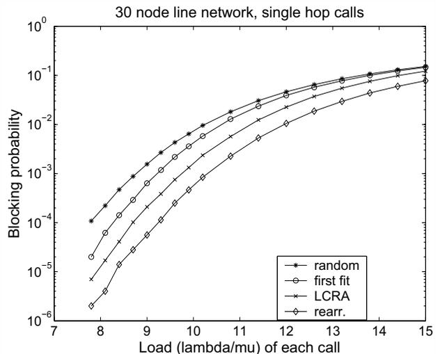
Fig. 9. Line network with unit length calls.
