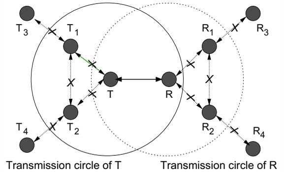
Fig. 1. Interference model for a bi-directional transmission ( $T \leftrightarrow R$ ).
