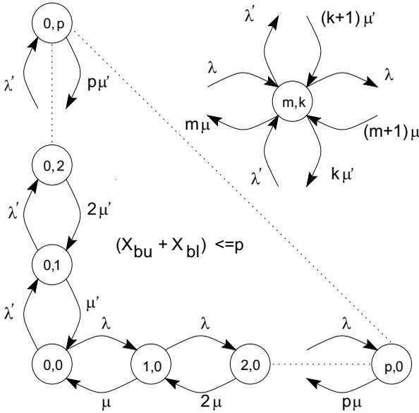
Fig. 4. State transition diagram for the random assignment policy.
