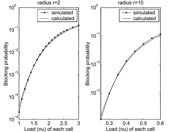
Fig. 6. Comparison of theoretical and simulated values for random policy,  $r = 2, 10$  and  $p = 20$  channels.
