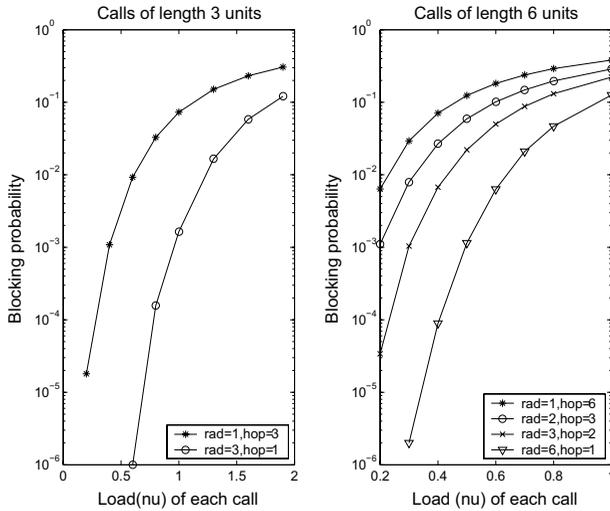
Fig. 7. Line network with calls of length 3 and 6 and 20 channels.
