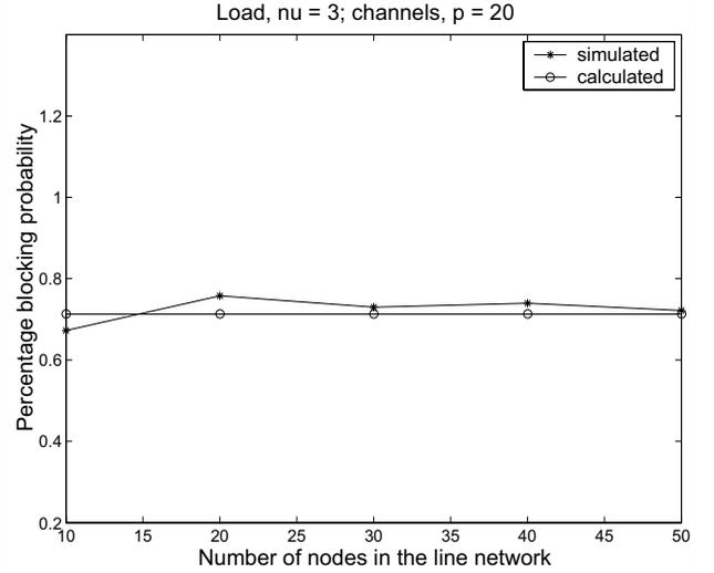
Fig. 5. Comparison of theoretical and simulated values for random policy,  $r = 1$ ,  $\nu = 3$  and  $p = 20$  channels.
