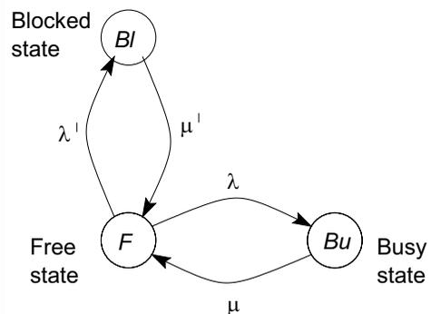
Fig. 3. Three state Markov process model of the channel on a link.
