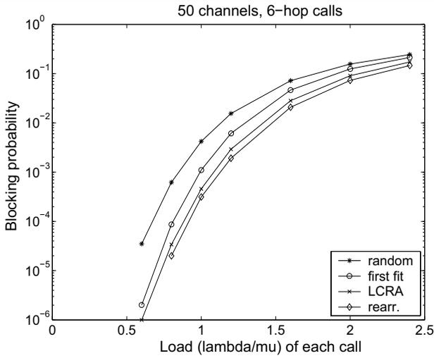
Fig. 11. Line network with 6-hop calls (length 6 units).
