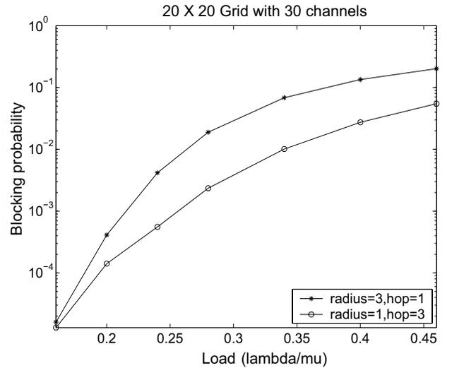
Fig. 8. Grid network with calls of length 3.
