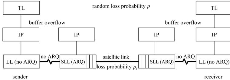
Fig. 1. System with two nodes communicating over a hybrid space-terrestrial network.
