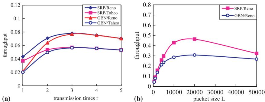
Fig. 6. Throughput versus SLL transmission times and packet size.
