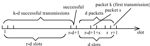
Fig. 3. Transmission pattern for SRP when  $k > d$ .
