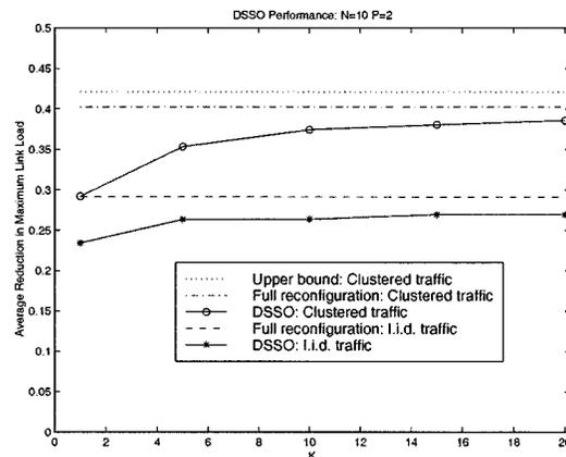
Fig. 6. Time average maximum link load reduction resulting from DSSO reconfiguration as a function of  $K$ , the number of steps between independent random traffic patterns. Results are for a network with  $N = 10$  nodes and  $P = 2$  ports per node.
