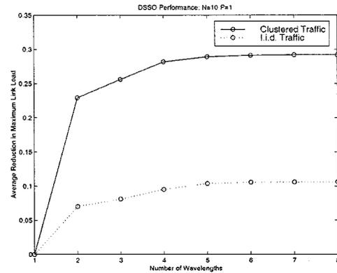
Fig. 7. The average reduction in maximum link load achieved by the DSSO reconfiguration algorithm is plotted as a function of the network wavelength restriction for dynamic traffic with  $K = 10$ . Results are for a network with  $N = 10$  nodes and  $P = 1$  port per node.
