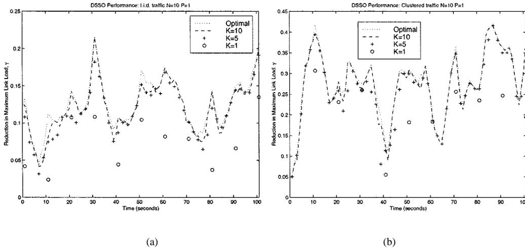
Fig. 3. Reduction in maximum link load achieved with DSSO algorithm and optimal reconfiguration strategies under dynamic traffic on a network with  $N = 10$  nodes and  $P = 1$  port per node. (a) I.i.d. traffic. (b) Clustered traffic.
