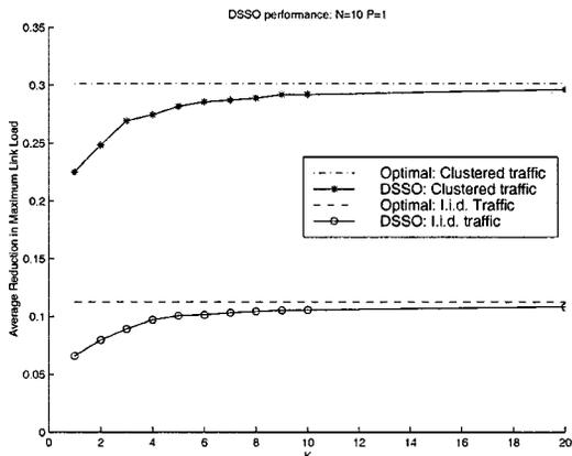
Fig. 4. Time average reduction in maximum link load resulting from DSSO reconfiguration as a function of  $K$  the number of steps between independent random traffic patterns. Results are for a network with  $N = 10$  nodes and  $P = 1$  port per node.
