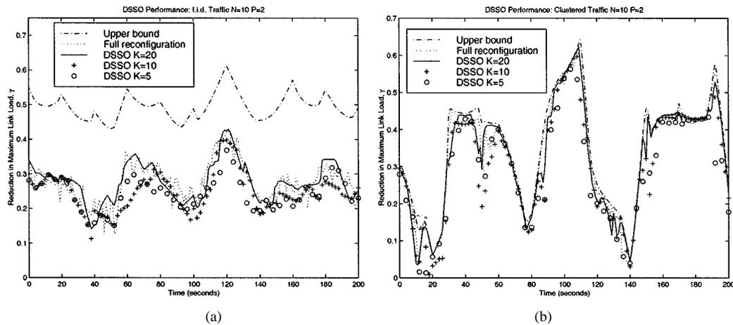
Fig. 5. Reduction in maximum link load achieved with DSSO algorithm under dynamic traffic conditions on a network with  $N = 10$  nodes and  $P = 2$  ports per node. (a) I.i.d. traffic. (b) Clustered traffic.
