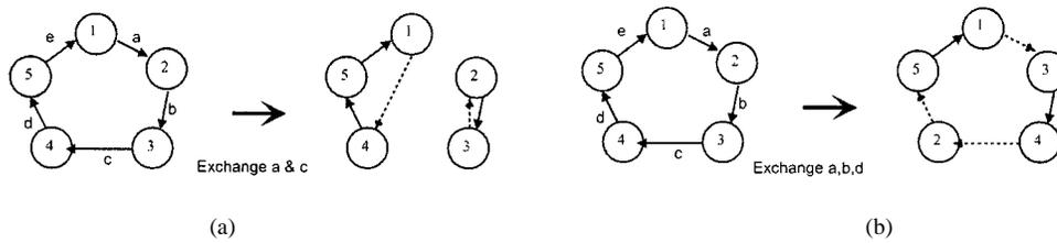
Fig. 1. Local exchange approaches applied to a ring topology. (a) 2-branch exchange. (b) 3-branch exchange.
