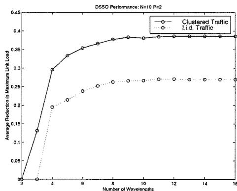
Fig. 8. The average reduction in maximum link load achieved by the DSSO reconfiguration algorithm is plotted as a function of the network wavelength restriction for dynamic traffic with  $K = 20$ . Results are for a network with  $N = 10$  nodes and  $P = 2$  ports per node.
